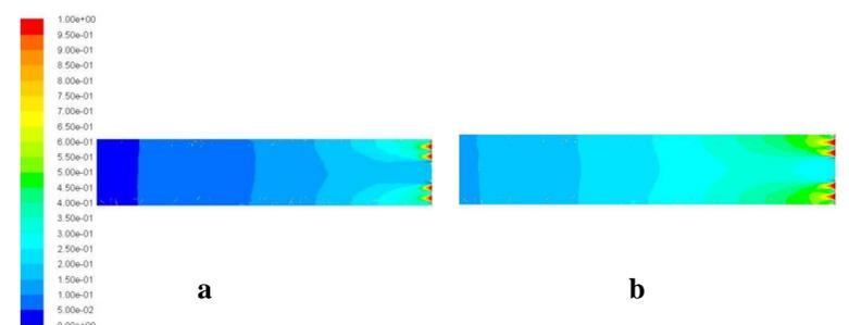
Figure 3. Contours of mass fraction of pollution ( a -  $M_0$  mass flow rate ; b -  $2M_0$  mass flow rate); ozone flow rate in both case was the same
