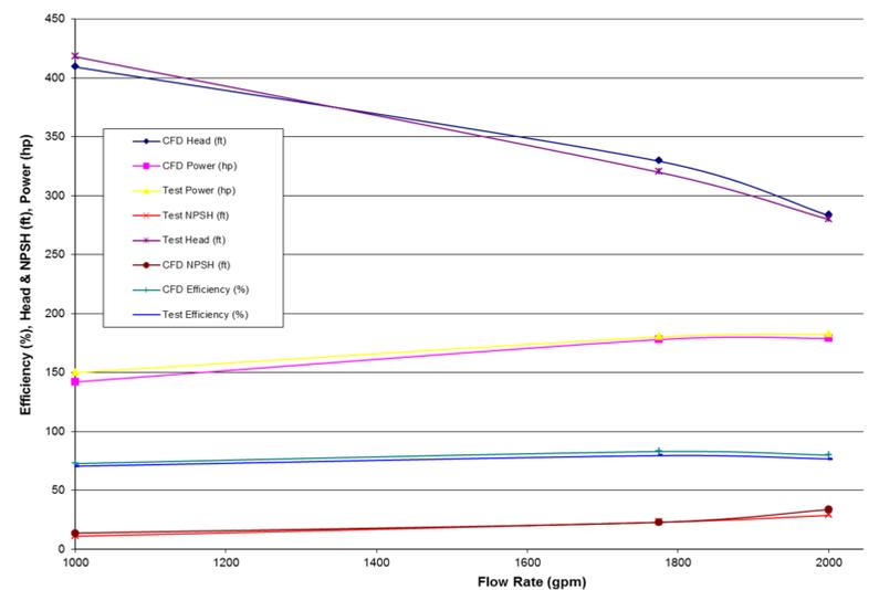
Figure 2. Comparison of CFD calculations for H, Efficiency and NPSHr vs. test data
