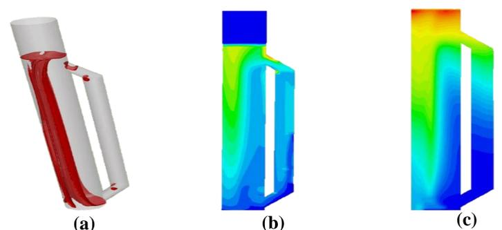
Figure 4. Water-air interface (a), bubble size distribution (b), oxygen concentration in (c)
