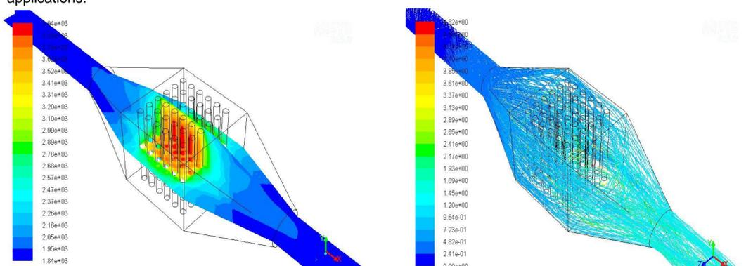
Figure 5(a). UV Radiation Field Strength (W/m2)
