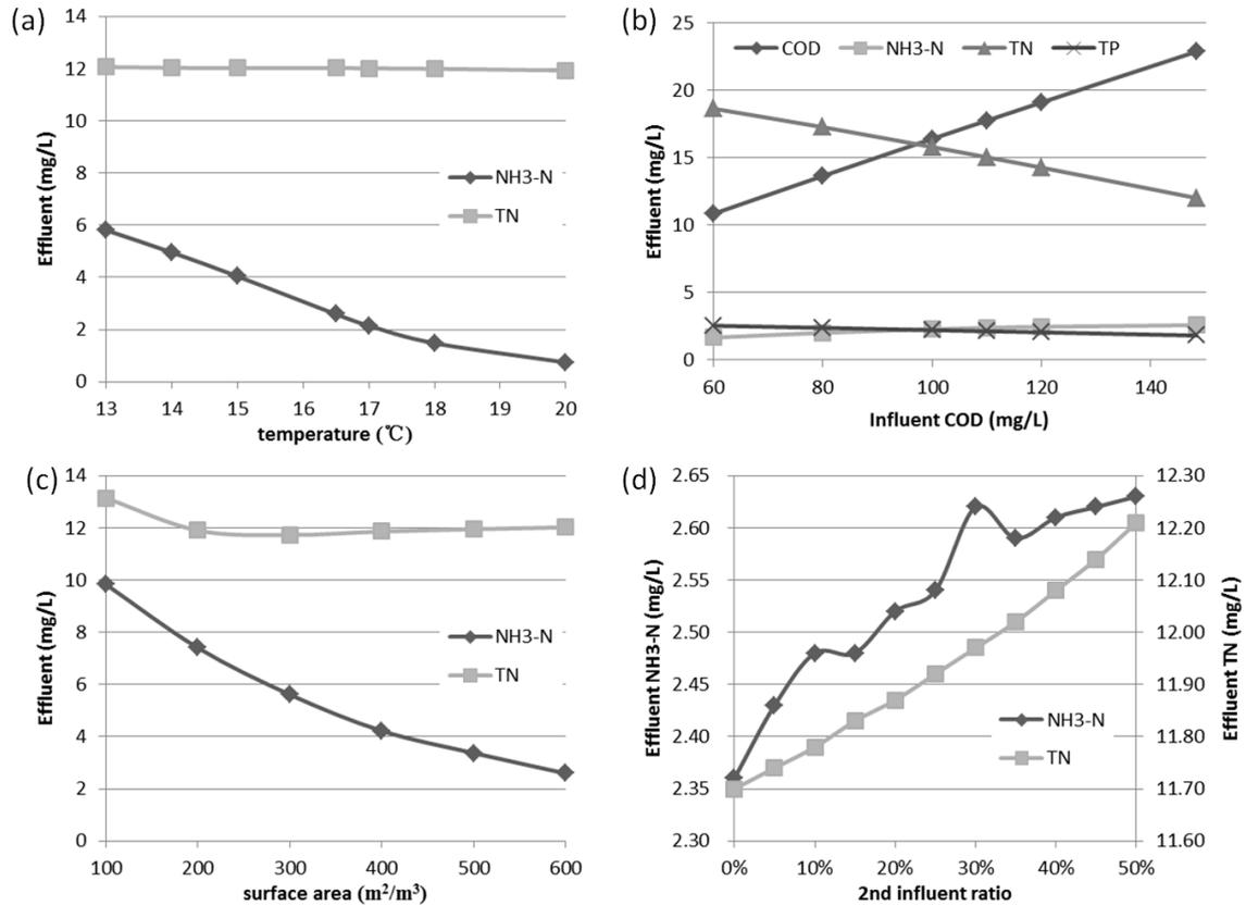
Figure 3 influence on (a)temperature, (b)influence COD, (c) surface area in MBBR, (d)2<sup>nd</sup> influent ratio in the reformed process
