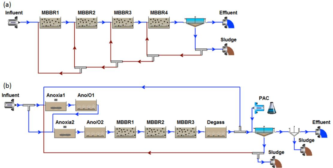
Figure 1 Model of WWTP (a) current process (b) reformed process
