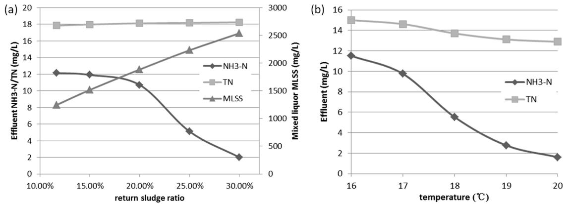
Figure 2 influence on (a) return sludge ratio, (b) temperature when 1# anoxic in current process
