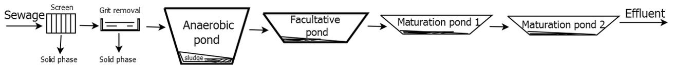
**Figure 1.1 A schematic showing a typical waste stabilization pond system**
