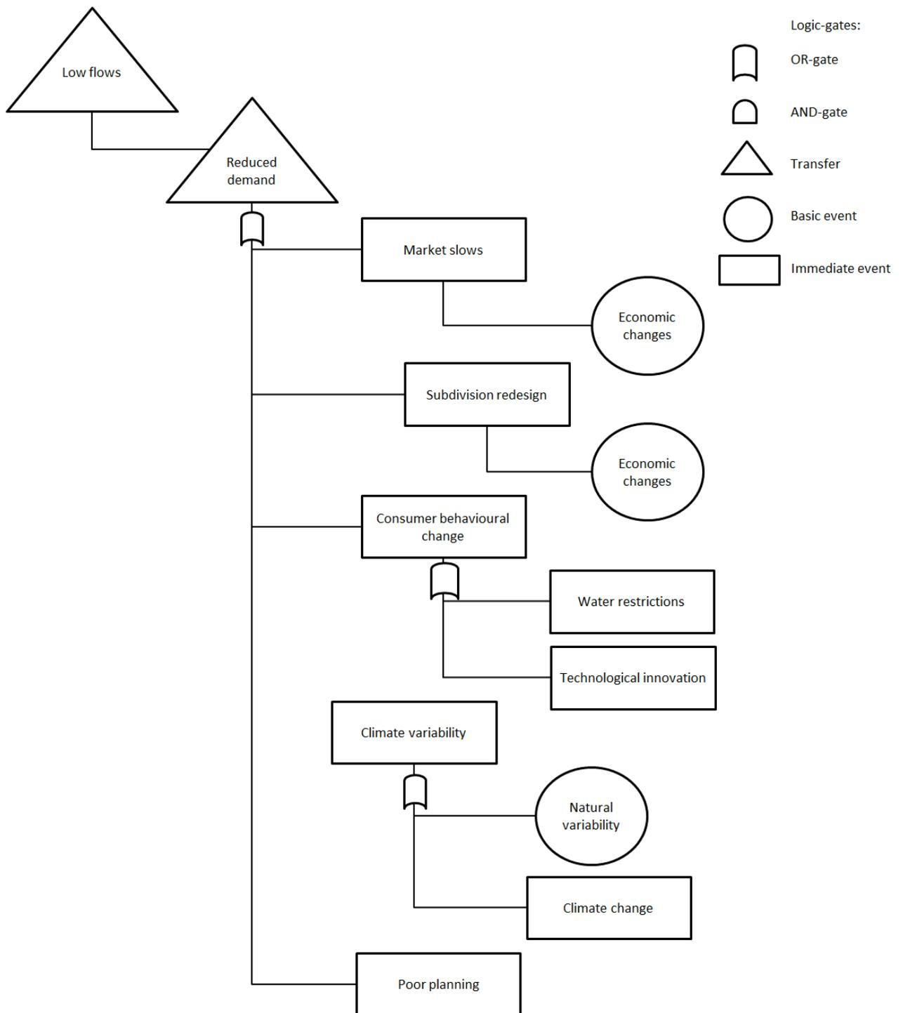
Figure 1.1 Fault tree of events leading to reduced demand from non-potable urban water schemes
