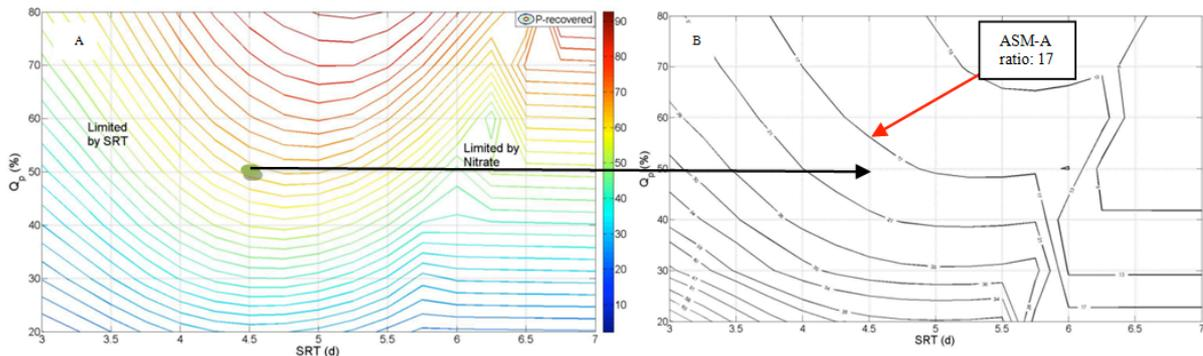
**Figure 2 a) Process performance as the N to P molar ratio fed to the downstream PBR as a function of the P-stream flow and the SRT; b) process performance as a percentage of P recovered from the influent as a function of the P-stream flow and the SRT.**
