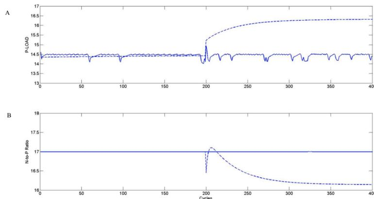
**Figure 3 Effect of a step change of 20% on the influent phosphorus: a) P-load in the P-stream; b) N-to-P ratio in the EBP2R effluent. In full line is presented the process response under controlled conditions and in dashed lines the process response without control. The step is introduced in cycle 200 (50 days).**
