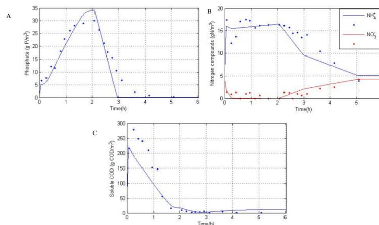
**Figure 1 SBR cycle performance: a) phosphate concentration; b) ammonia and nitrate concentrations; c) soluble COD concentration. Dots represent the experimental data, while the full line represents the simulated results.**
