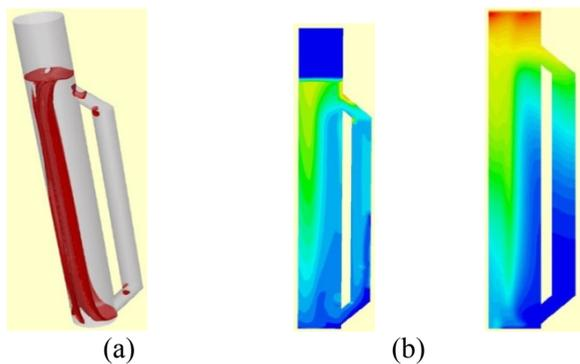
Figure 2. Water-air interface (a), bubble size distribution (b) and Oxygen Concentration in (c)
