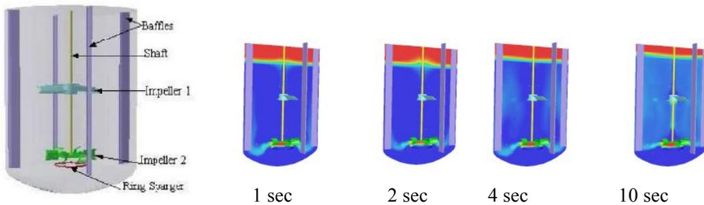
Figure 1(a). Figure 1(a). Air Volume Fraction in a tank from zero (blue color) to 1 (red color)
