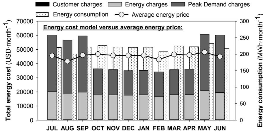
Figure 1 Evaluation of the energy costs by using: i) the Real energy cost model (bar plot) and ii) an average energy price of 0.207 \$/kWh (line plot). The total energy consumption is given on the right axis.
