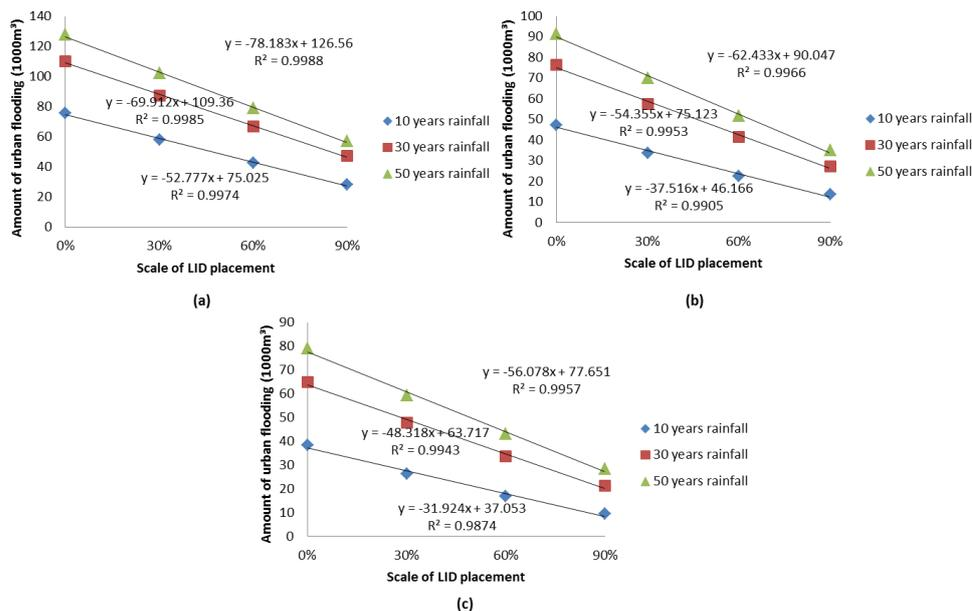
Figure 2 Amount of urban flooding for rainfalls of different return periods: (a) 1 year drainage system; (b) 3 years drainage system; (c) 5 years drainage system
