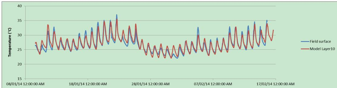
Figure 1.1 A comparison of measured and simulated temperature data at the water surface level
