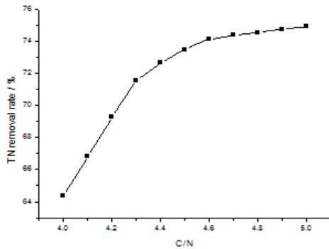
**Figure 2. TN removal rate of simulation**
