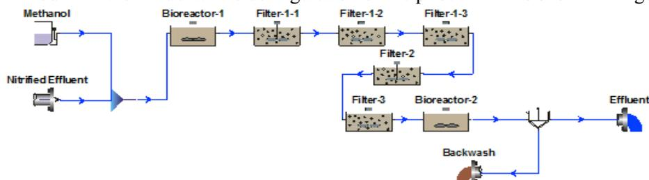
**Figure 1.** General model configuration of pilot DNBf
