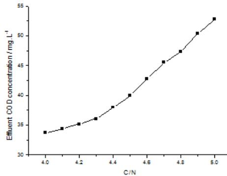
**Figure 3. COD conc. of effluent by simulation**
