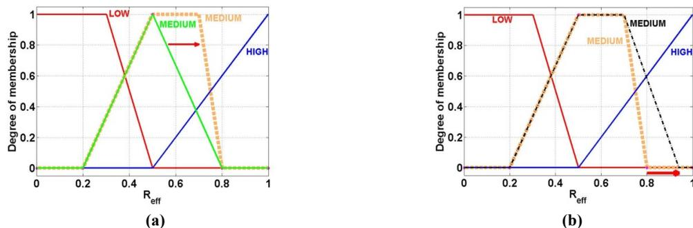
**Figure 1.1:** (a) Increase of the MF slope for fuzzy subset “medium” of  $R_{\text{eff}}$ , and (b) increase of the crisp value to which 0 degree of membership to fuzzy subset “medium” corresponds.
