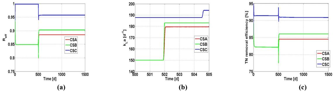
**Figure 1.2:** Dynamic simulation results for Scenario 1: (a) ammonium removal efficiency ( $R_{eff}$ ), (b)  $k_{La}$ , and (c) total nitrogen removal efficiency.
