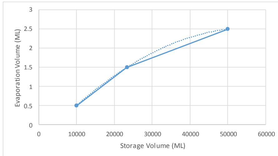
Figure 2. Example evaporation curve with three points in the linearized approximation.
