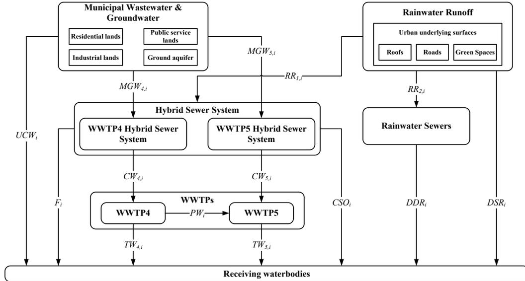
Figure 1 Framework of NK-UDS and substance flow paths
