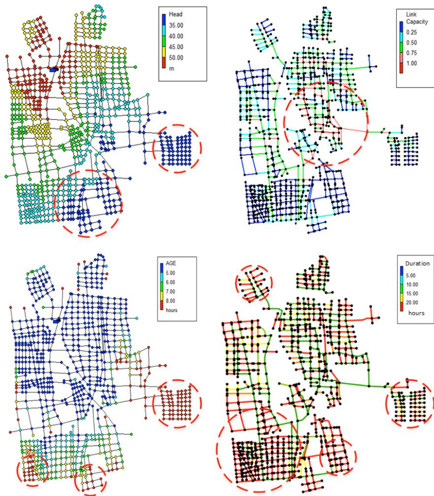
Figure 2 The hydraulic performance of water network system. (a) Water head and (c) Water age in the water distribution system; (b) Depth to diameter ratio and (d) Duration with a lower velocity than the self-cleansing one, i.e. 0.6 m/s, in the sewage system.
