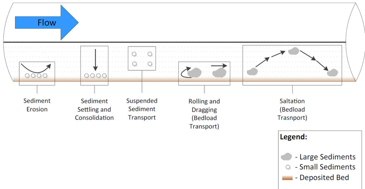
**Figure 1.2 Sewer sedimentation processes**
