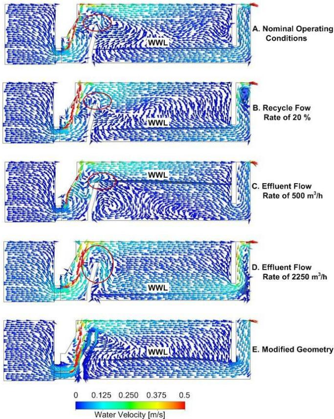
Figure 3. Water Velocity Vectors and White Water Level.
