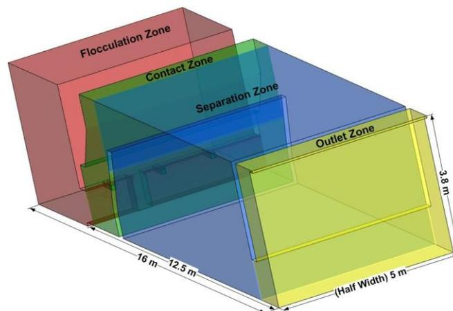
**Figure 1.** DAF Tank dimensions and zones.
