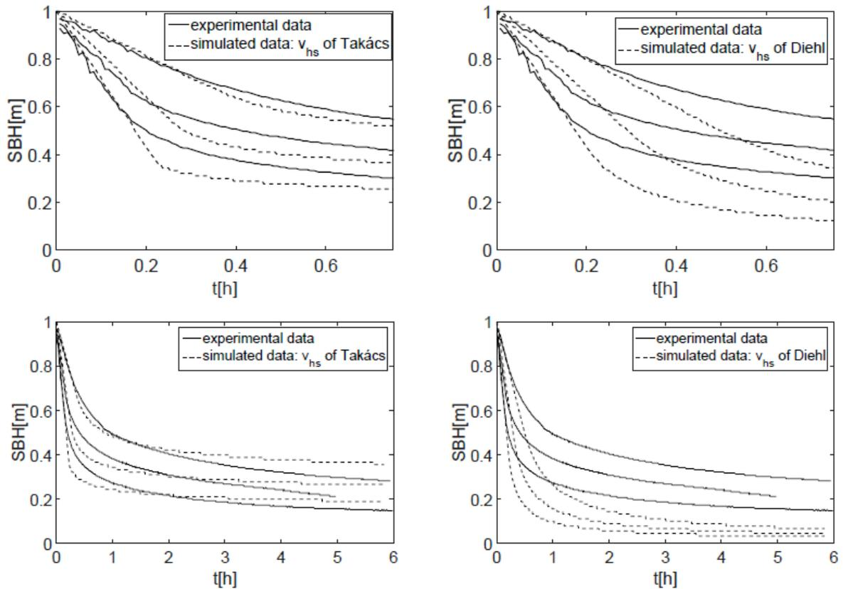
**Figure 2: Measured sludge blanket heights (solid line – from De Clercq et al. (2005) and predicted sludge blanket heights (dashed lines) by the Bürger-Diehl model with only hindered settling. Left: hindered settling function of Takács, right: hindered settling function of Diehl (2014).**
