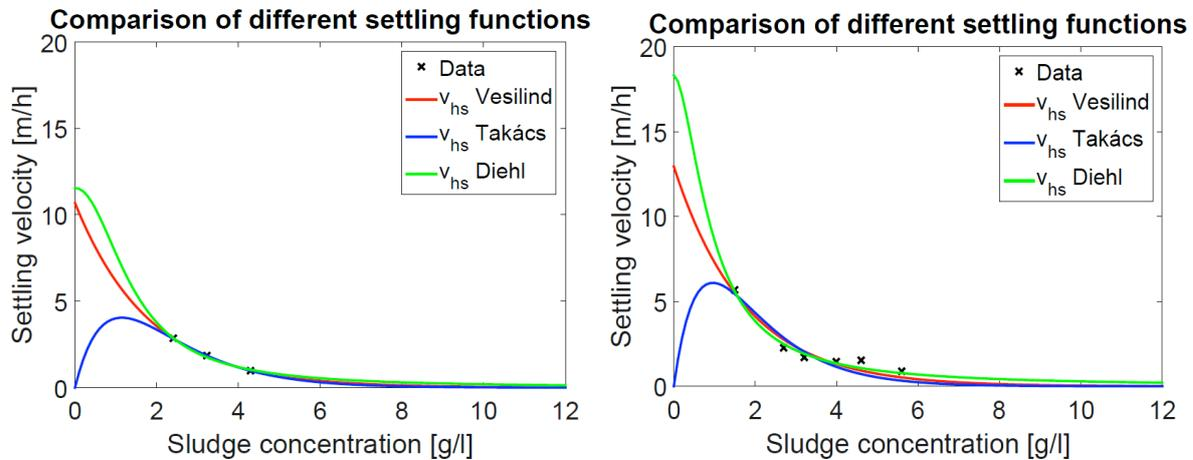
**Figure 1: Comparison of different hindered settling functions against measured data of De Clercq et al. (2005) (left) and data of Locatelli et al. (2014) (right).**
