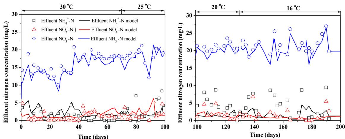
Figure 1 Model calibration using the measured effluent nitrogen concentrations in the initial 99 days of operation under ambient temperature of 30-25 °C (A); Model validation using the measured reactor effluent concentrations between 100 and 200 days operation under low temperature of 20-16 °C (B).
