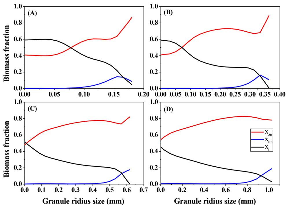
**Figure 2 Biomass distribution at various granule sizes (A: granule radius size of 0.18 mm; B: granule radius size of 0.365 mm; C: granule radius size of 0.62 mm; D: granule radius size of 1.185 mm. Note: Radius in the figure is surface area-weighted mean radius.)**
