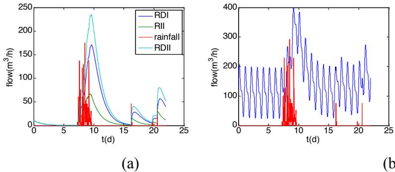
Figure 2 (a) The RDII process for each rainfall event, and (b) The total flow in the sanitary sewer.
