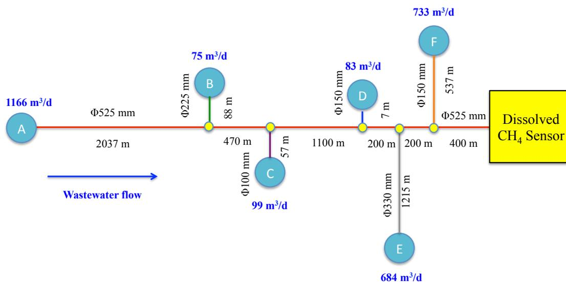
Figure 1. Details of the sewer network and the sensor location
