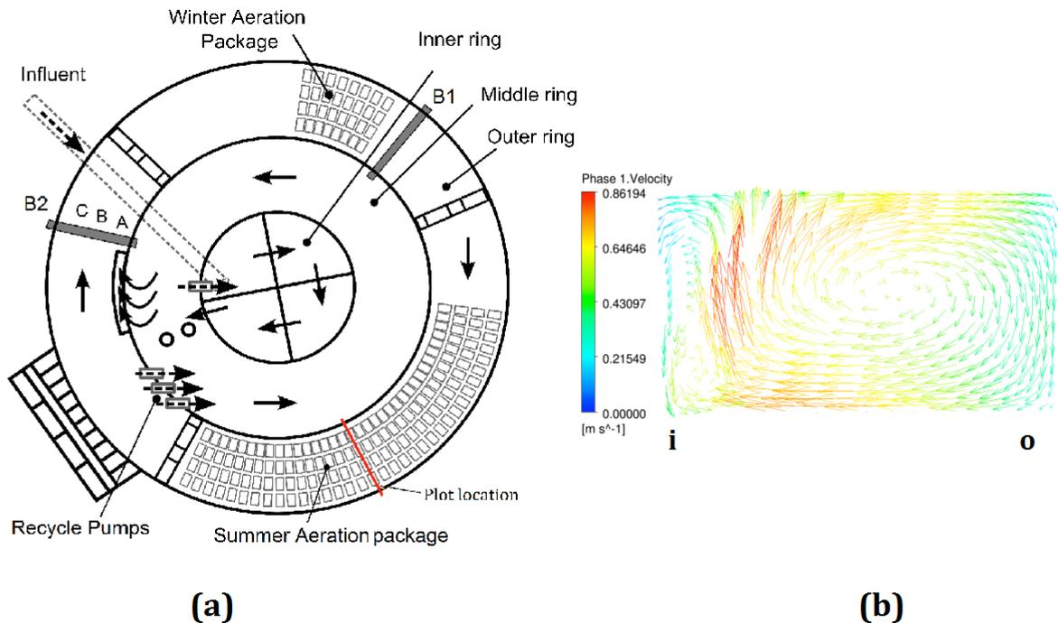
**Figure 1** (a) Flow configuration of the bioreactor, (b) Velocity vector plots at the vertical cross section in the aerated region
