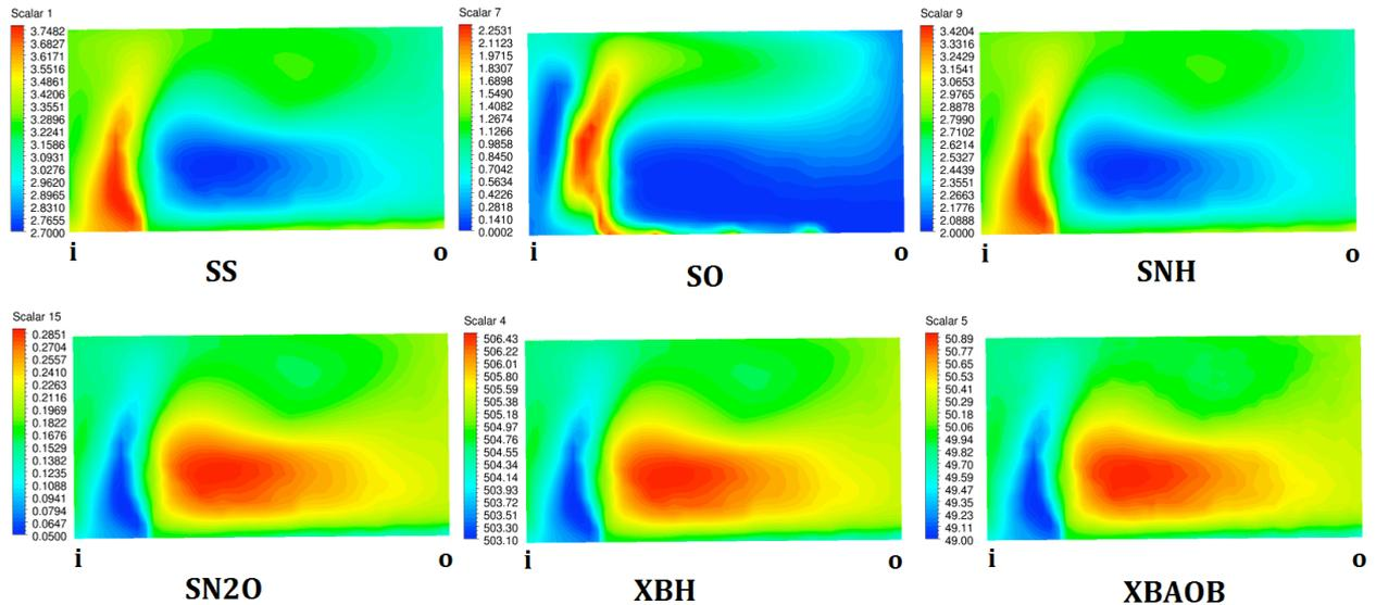
**Figure 2 Contour plots for different components (mg/L)**
