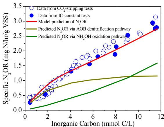
**Figure 2.** Model evaluation results using experimental data from the nitrifying culture.
