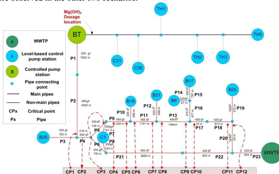
Figure 1.1 The scheme of the Tugun-Elanora sewer network
