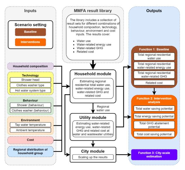
Figure B-1: Overview Model concept being developed for the Net Zero Water Cycle Project.
